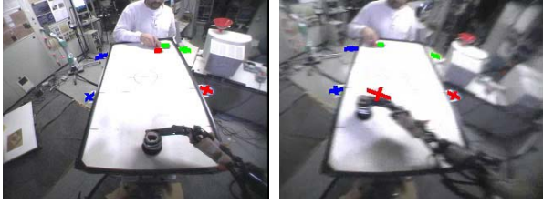
Figure 4: The view from the robot's eyes with the tracked objects marked. The puck is totally occluded in the right image. The right image is also blurred due to the movement of the robot.
